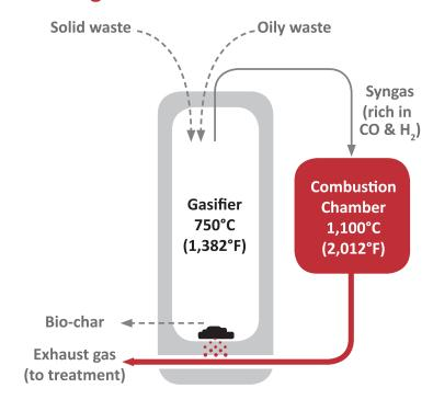
Auto Gasification is Terragon's patented technology. It thermally breaks down waste into bio-char and syngas, which it uses to make the process self-sustaining.
